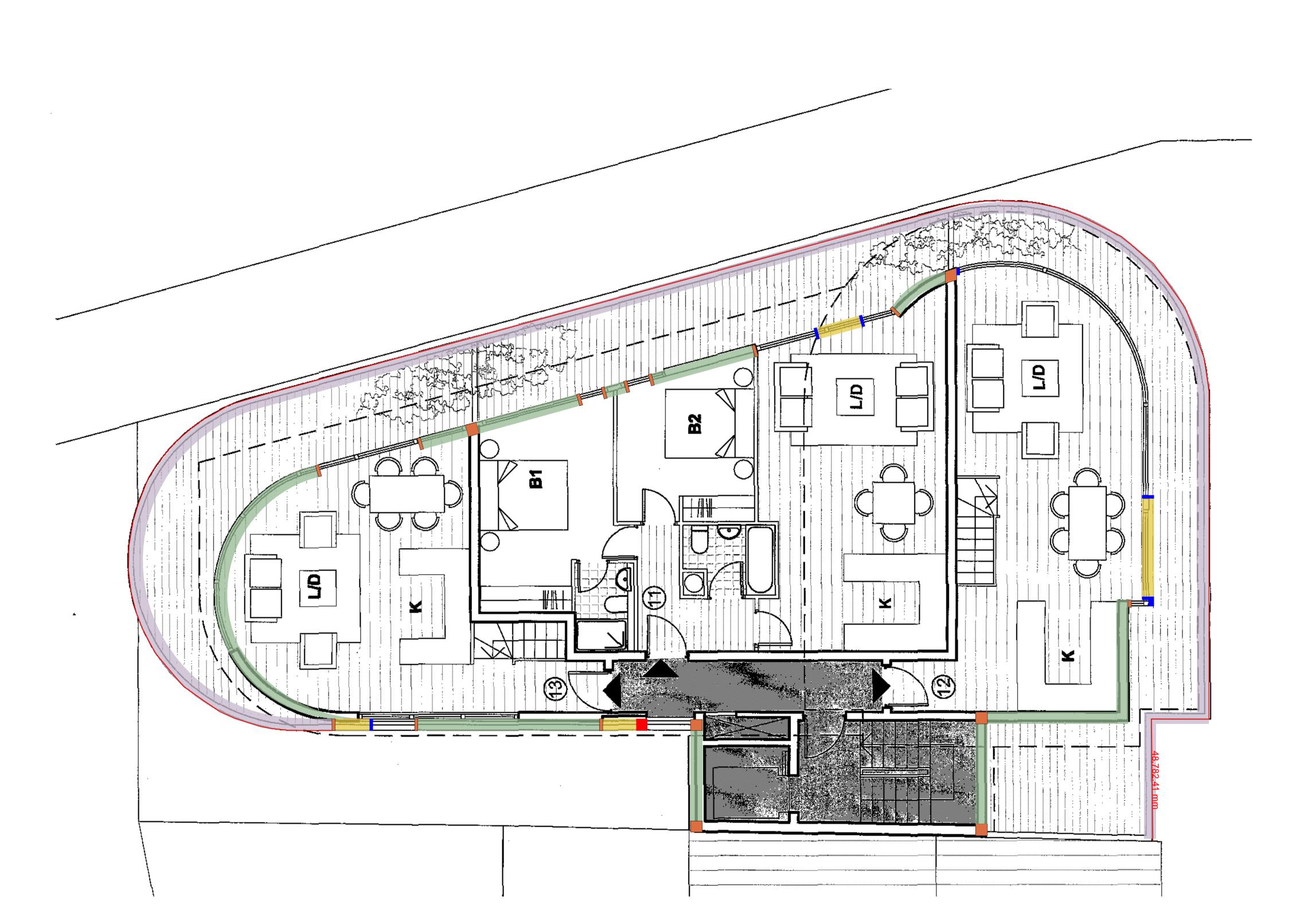
Cavity Barrier 30min Integrity/15min Insulation (tbc Marshalls)
